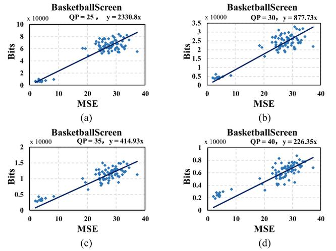
Fig. 6. The R-MSE curves for scene unchanged frames under different QPs.
