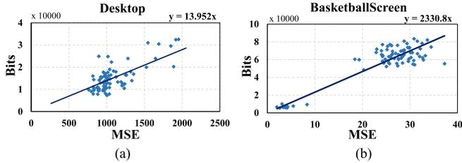
Fig. 5. The R-MSE curves of scene unchanged frames.
