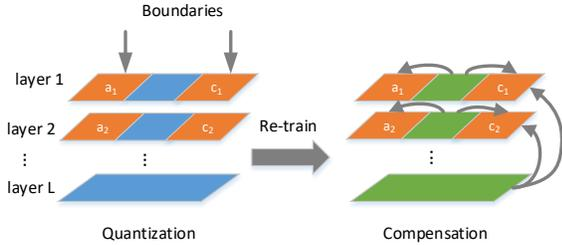
Figure 5: Quantization process of multi-level ternary quantization. Blue, green and orange parts indicates the full precision, re-trained and quantized layers. We first quantize the Boundaries and then quantize the Hearts of the network.
