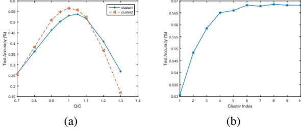
Figure 3: (a) shows the quantization of two different clusters generated by k-means in AlexNet.  $Q/C$  means the value  $Q$  that weights to be quantized into is divided by the centroid of the cluster  $C$ . The accuracy of the network changes with the change of  $Q$ . (b) shows the test accuracy when 10 clusters of AlexNet are quantized respectively. The clusters are sorted in the descending order.
