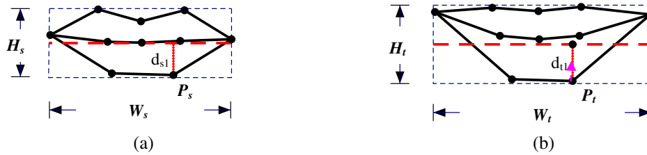
Fig. 3. Local re-shaping process of the mouth in vertical direction (the feature point P_t is moved vertically to make the height-to-width ratio of (b) close to (a)). (a) The mouth feature positions of the source person's expression face, (b) the mouth feature positions of the globally warped target person expression face (the blue dashed box is the minimum bounding box surrounding the mouth feature positions and the red dashed line is the horizontal middle line of the minimum bounding box). (For interpretation of the references to colour in this figure legend, the reader is referred to the web version of this article.)
