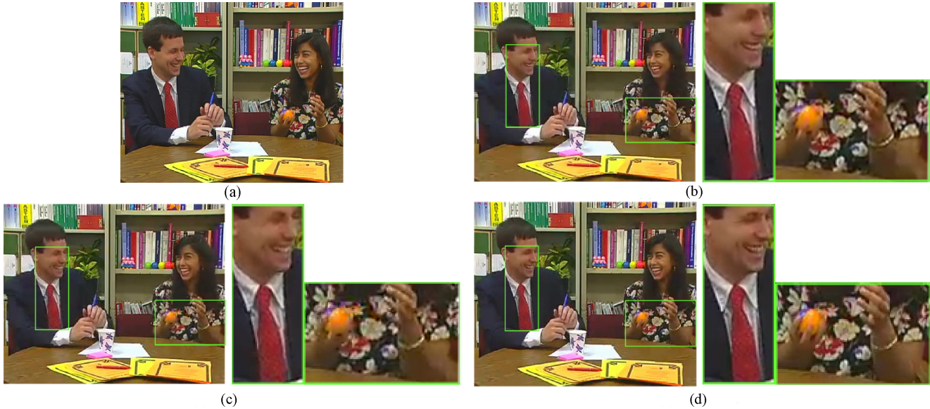
Fig. 8. Comparison of the subjective visual quality of the 38th frame of Paris at CIF 128 kb/s. (a) Original. (b) Frame layer (FL). (c) RBUR T1. (d) RBUR T2.
