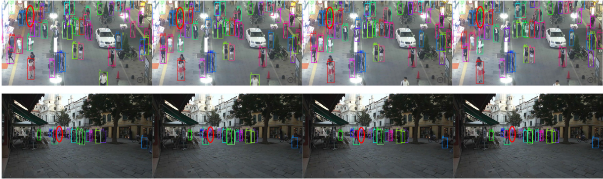
Fig. 12. Some failure cases (highlighted with red circles) when performing tracklet-plane matching on MOT17 test datasets. (For interpretation of the references to colour in this figure legend, the reader is referred to the web version of this article.)
