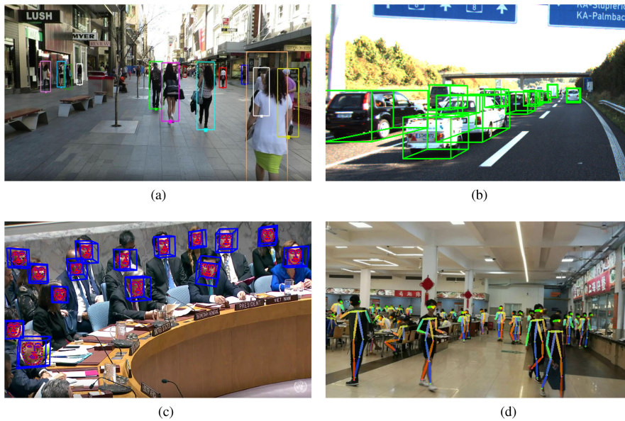
Figure 3. Examples of different key points. Best viewed in color. (a) 2D bounding boxes. (b) 3D bounding boxes. (c) Facial landmarks. (d) Skeletons.
